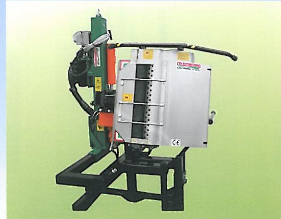
MACCHINA A RIPOSO SU TELAIO REVERSIBILE CON INCLINATORE AUTOLIVELLANTE E MASCHERINA ANTI-INTRUSIONE TRALCI
